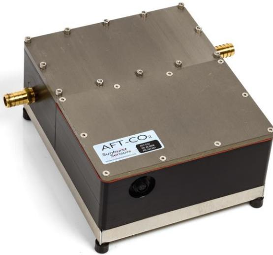
*Sunburst Sensors flow-through  $p(\text{CO}_2)$  system.*
