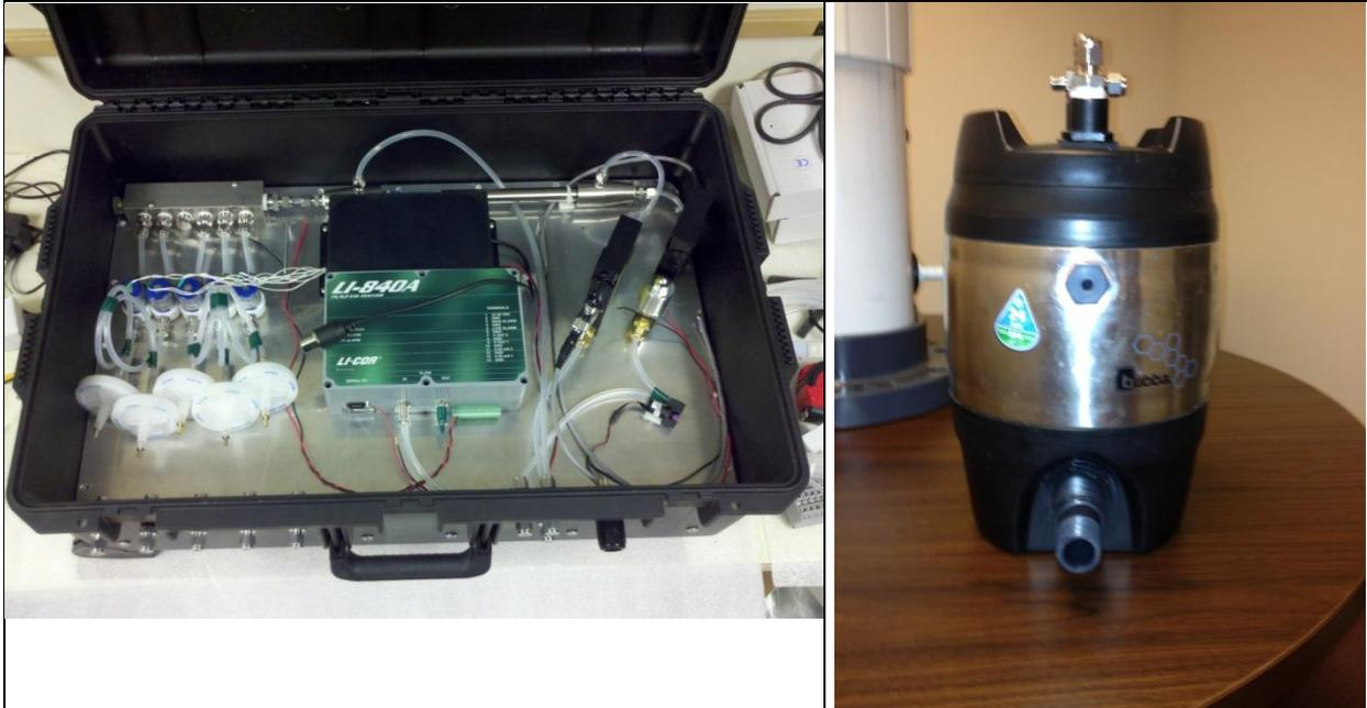
*Left, an inside view of the Licor™ based pCO<sub>2</sub> monitoring system built by University of New Hampshire's Coastal Carbon Group. Right, the shower head equilibrator built into a small commercial Bubba™ cooler.*
